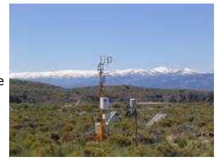
Measuring tower of CO2 ecosystem-atmosphere interchange by means of the eddy covariance technique.
