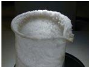
Salt crystals can have very abrasive effects on stone and other building materials.
